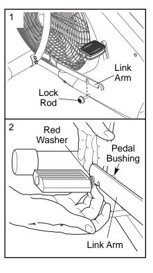
gers as shown. **Be careful not to pinch your fingers.** Next, slide the link arms onto the pedal bushings. Move the link arms up and down slightly to make sure that they are fully seated on the pedal bushings. **CAUTION:** Make sure that the link arms are fully seated on the pedal bushings. If the link arms are not on the pedal bushings, they may slip off during use, resulting in injury to the user.
